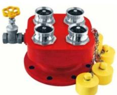
Fire Brigade Inlet (also called Pumping In Breech) allows Fire Tenders (Pumpers) to pump in water into the Dry Riser/ Wet Riser/ Sprinkler system piping using external water sources such as hydrants. Fire Brigade Inlet is fitted with required number of standard Male Instantaneous inlets to feed the Riser pipe depending upon size.
